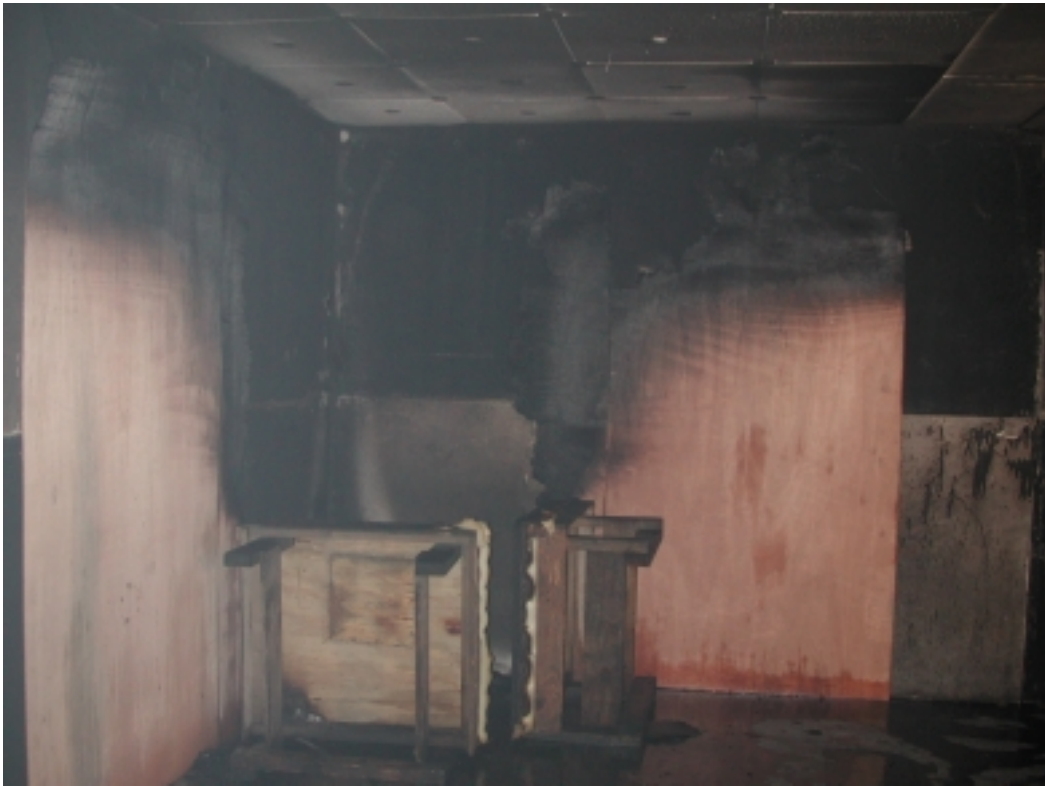
Figure A-9 The luxury cabin after the test.
