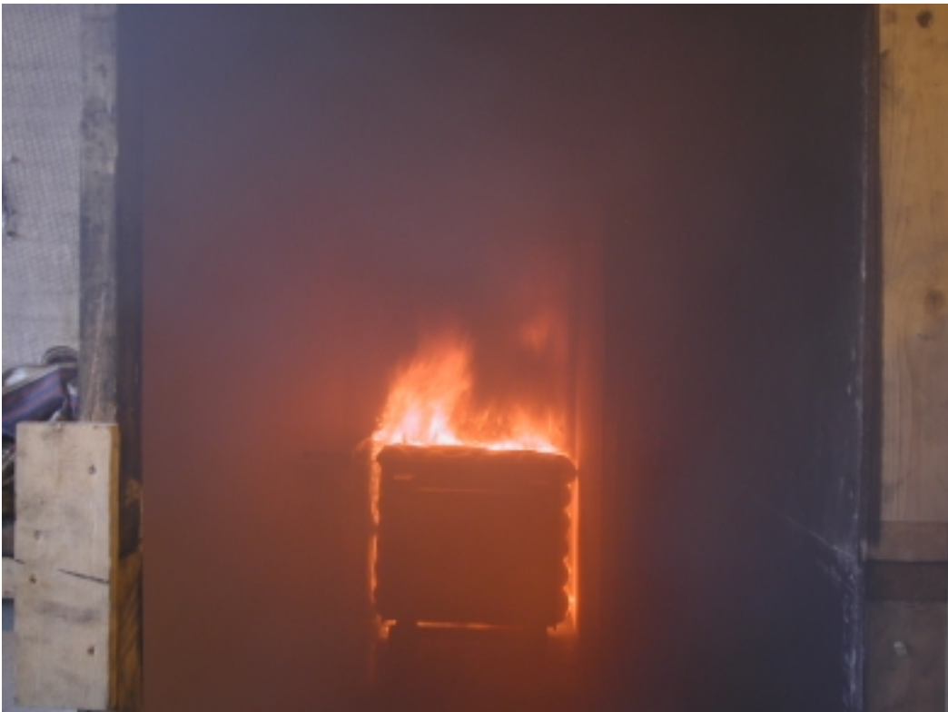
Figure A-8 The fire size at the activation of the first nozzle.
