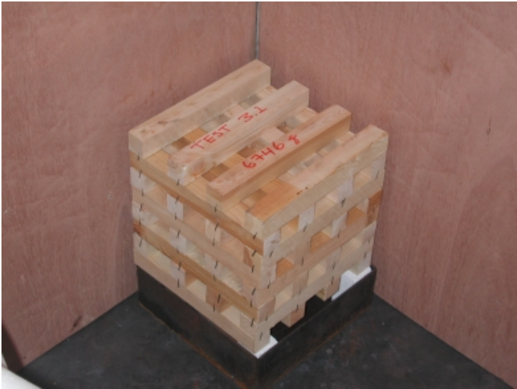
Figure A-5 Close up picture of the wooden crib positioned on top of the pan with n-heptane.
