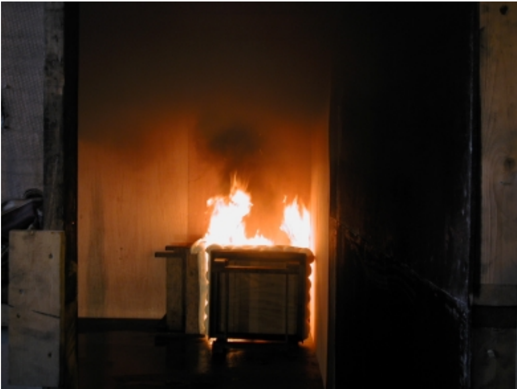
Figure A-7 The fire size prior to the full fire involvement of the polyether foam cushions.
