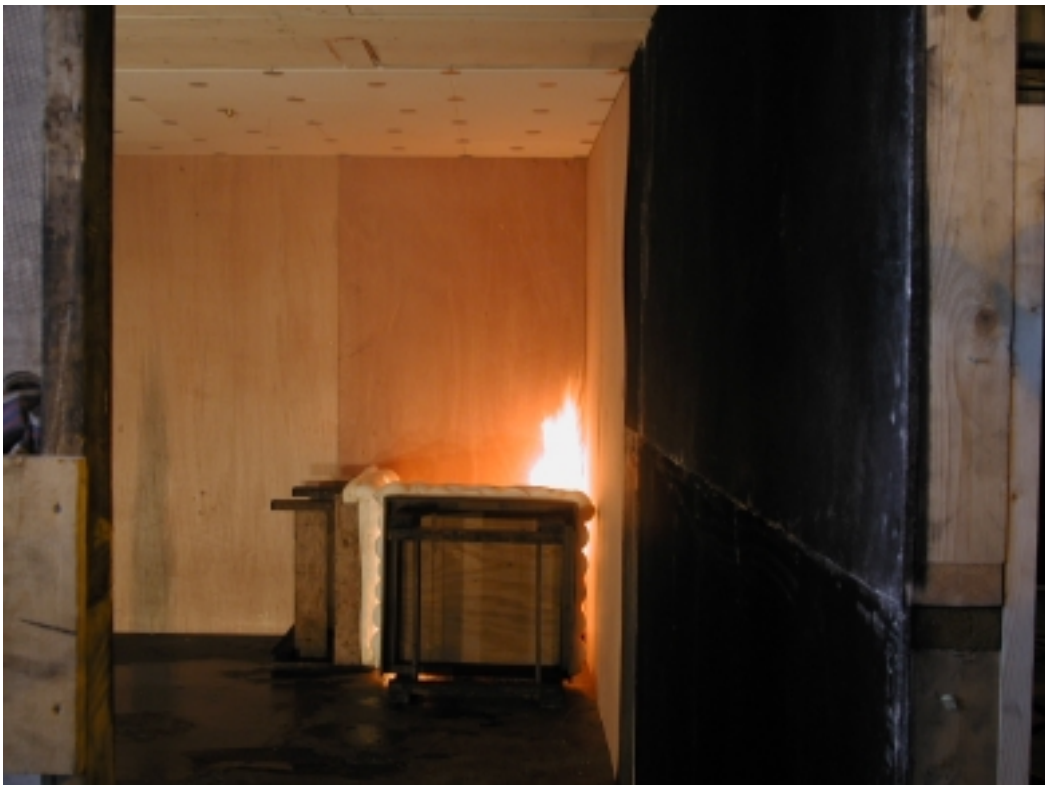
Figure A-6 The fire size slightly after the ignition of the excelsior (wood wool).
