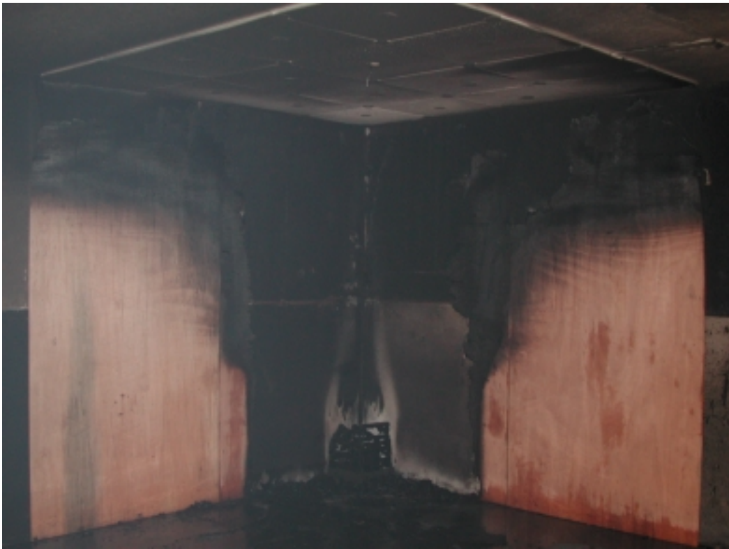
Figure A-10 The luxury cabin after the test, with the 'simulated furniture' removed.
