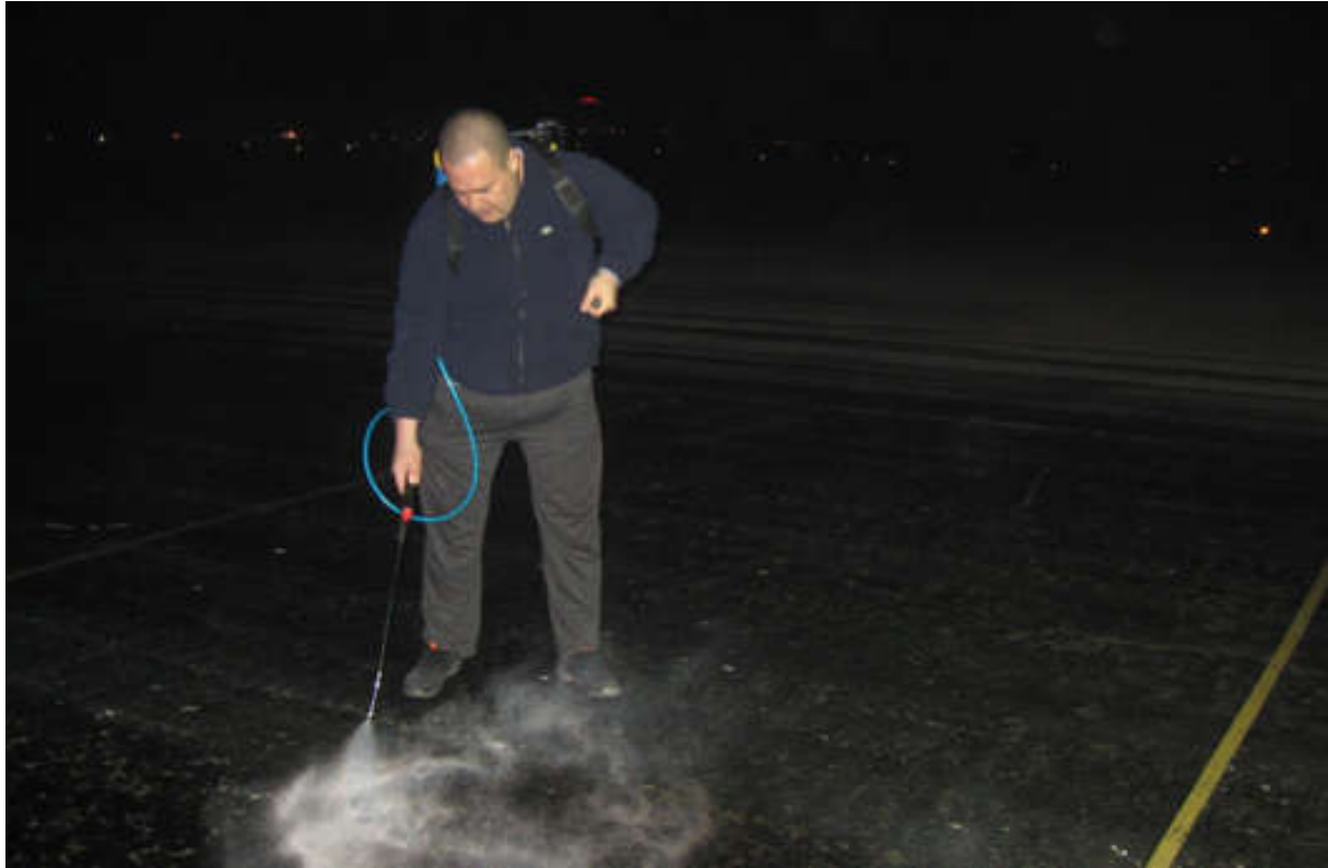
Picture 18 - Step 2 The application of the solvent solution: 00:45
